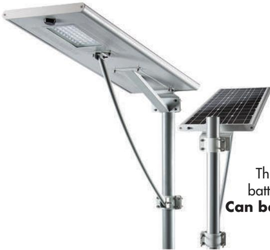
50W LED (110lm per Watt), 29Ah 12V Battery, Solar Panel 70W/18V, \*7hour Charge Time, Work Temp -30°C to 60°C, Aluminium Alloy + PC Lens, IP65,
